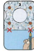
Mark the prestressing steel
