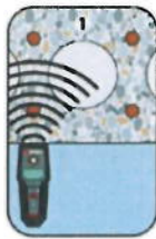
Locate the prestressing steel
